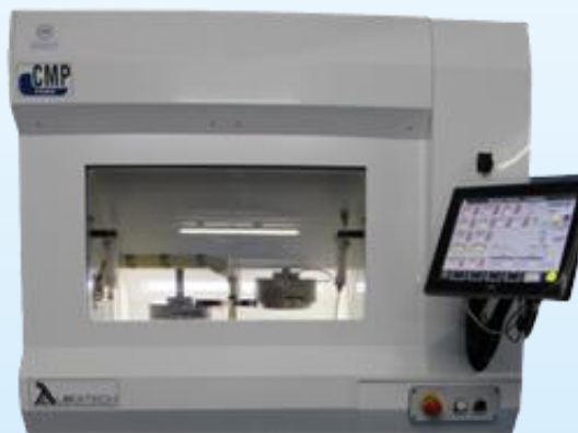
Wafer Planarization (Upto 100 mm wafer)
