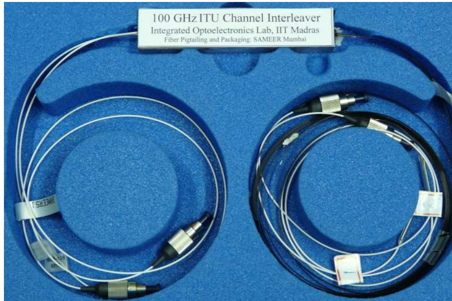
Figure 4.3: Photograph of a packaged prototype DWDM channel interleaver. Packaged device: GI12.
