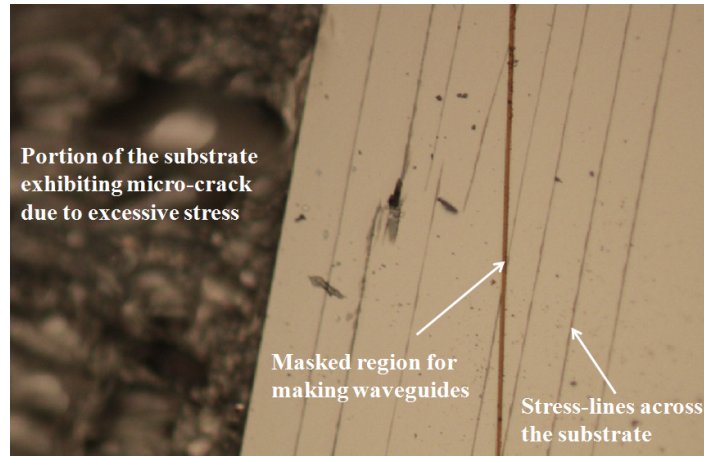
Figure 4.4: Surface damage in LiNbO 3 substrate during surface activation.
