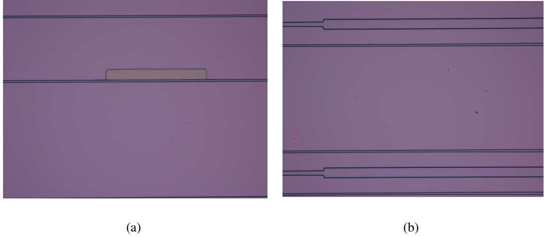
Figure 3.8: Microscopic views of a SOI sample just after phosphorous diffusion. The brownish-violet colour shows a layer of phosphosilicate formed over the sample's surface: (a) the SOI sample showing diffusion window of a p-i-n waveguide, (b) the SOI sample showing waveguides and input section of a MZI.
