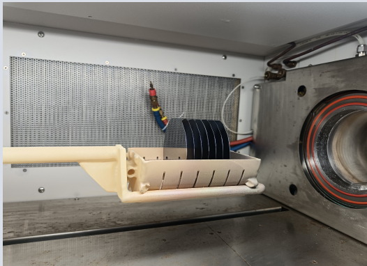
Loading of thermal wafers in SiN furnace
